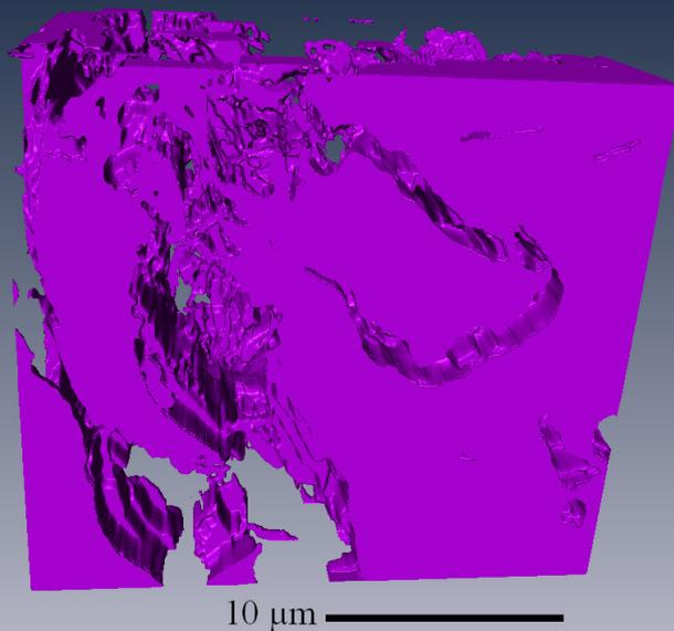
A 3D image of reactor core graphite in its irradiated state
